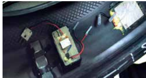
Car tires equipped with the power generation sheet and high efficiency storage circuits.
