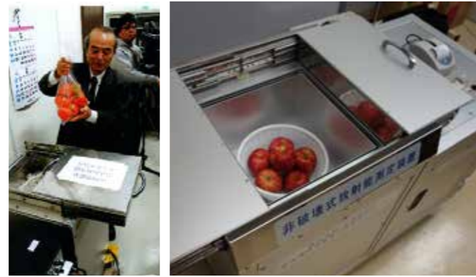
Development and installment of non-destructive radioactive contamination monitoring of food "as a whole".
