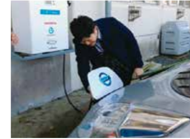
Energy supply utilizing an electric vehicle (EV) power station (V2H).
