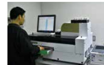
Radioactive Cesium Measurement with a gamma counter.
