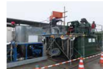
Separation of tsunami debris by the soil separator-multi method.
