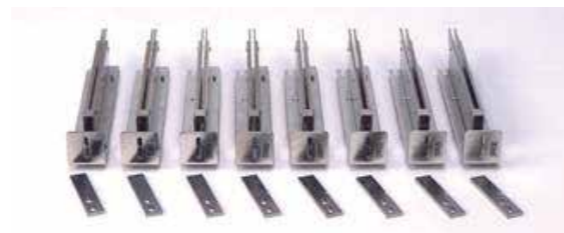
Rails used in the automatic screw feeder
