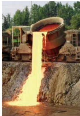
Steel slags after processing.
