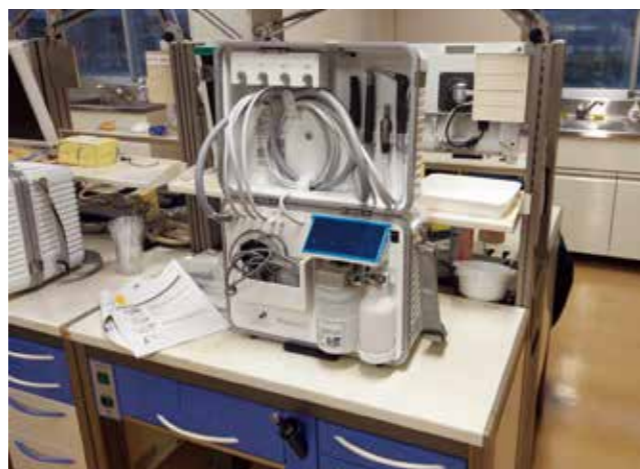
Portable dental unit: A suitcase-like mobile case that opens to become a dental treatment device.
